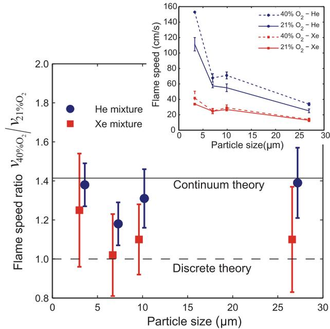
FIG. 4. (Color online) Ratio of flame speeds between two different  $O_2$  concentrations in He and Xe mixtures. The inset shows experimental measurements of the flame speed in iron suspensions in 21% and 40%  $O_2$  in He and Xe.
