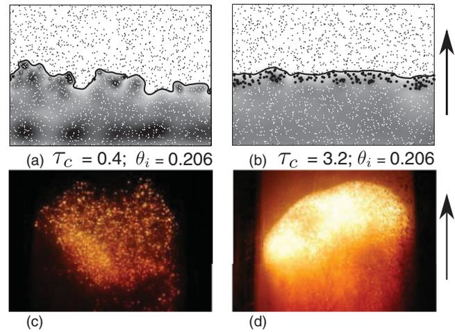
FIG. 3. (Color online) Two-dimensional numerical simulations and photographs of the flame in iron suspensions in Xe-O<sub>2</sub> [(a) and (c)] and He-O<sub>2</sub> [(b) and (d)] mixtures. The upward arrows indicate the propagation direction.
