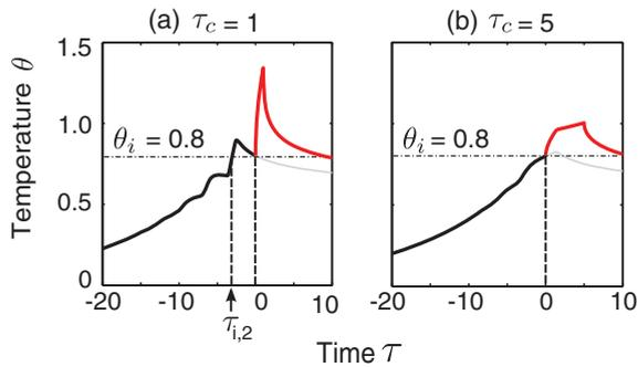
FIG. 2. (Color online) Time-temperature histories of a source igniting under physically (a) invalid and (b) valid conditions. The time  $\tau = 0$  corresponds to the ignition of the source and the thin gray line originating at  $\tau = 0$  corresponds to  $\theta$  if ignition is omitted. In (a), the first intersection between  $\theta$  and  $\theta_i$  is denoted as  $\tau_{i,2}$ .
