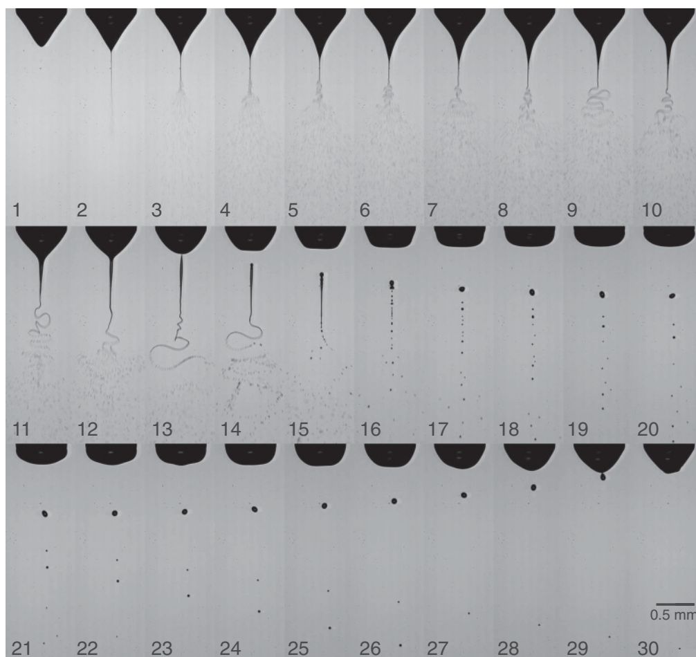
FIG. 2. Category C1 (complete coalescence): a droplet returns to the cone after being formed from a liquid ligament. The diameter of the returning droplet is \sim 80 \mu\text{m} , the time frame between images is \sim 45 \mu\text{s} , the applied potential is -5.67 \text{ kV} on the counter electrode, and the flow rate used is 1 \text{ mL h}^{-1} .
