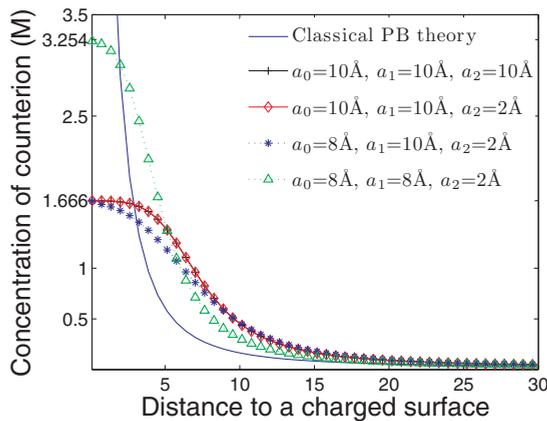
FIG. 4. (Color online) Counterion concentrations vs distance in Angstroms to the charged surface with different ionic sizes and with no ionic sizes (the classical PB theory). The linear size of counterions is  $a_1$ . The counterion concentration at the charged surface is  $1/a_1^3 = 1.666$  M when  $a_1 = 10$  Å and is  $1/a_1^3 = 3.254$  M when  $a_1 = 8$  Å.
