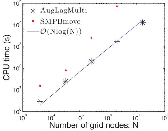
FIG. 3. (Color online) Log-log plot of the CPU time vs the number of grids for both SMPBmove and AugLagMulti.
