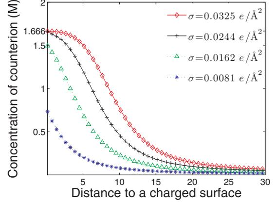
FIG. 5. (Color online) Counterion concentration vs the distance in Angstroms to the charged surface with different values of the surface charge density  $\sigma$ .
