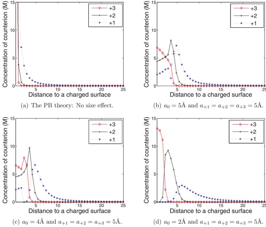
FIG. 6. (Color online) Concentrations of multivalent counterions vs the distance in Ångstroms to the charged surface. In the symbols,  $+i$  means the concentration of the counterion with the valence  $+i$  ( $i = 1, 2, 3$ ). (a) The classical PB solution: without the size effect. (b) The size effect included with the linear sizes of group I. (c) The size effect included with the linear sizes of group II. (d) The size effect included with the linear sizes of group III.
