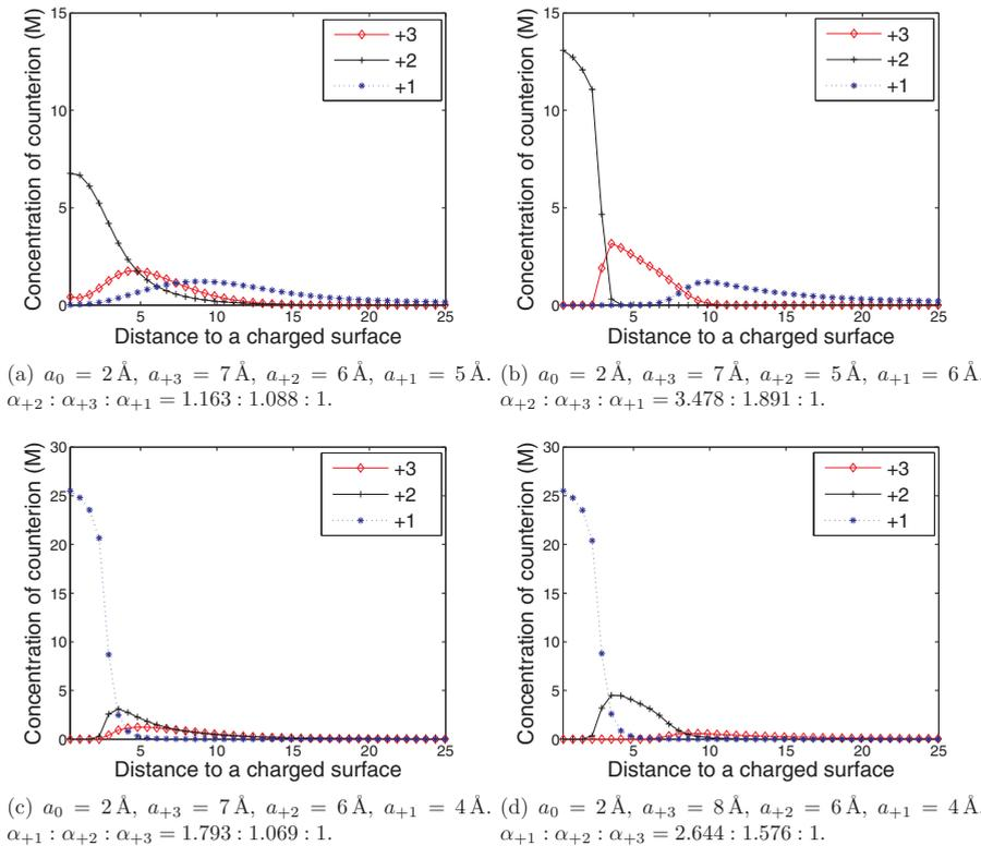
FIG. 7. (Color online) Concentrations of multivalent counterions vs the distance in Ångstroms to the charged surface. In (a) and (b),  $\alpha_{+2} > \alpha_{+3} > \alpha_{+1}$ . In (c) and (d),  $\alpha_{+1} > \alpha_{+2} > \alpha_{+3}$ .
