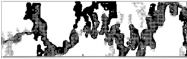
FIG. 6. The occupation of air in the experimental cell is shown by the solid black flow pattern (Fig. 5). The air occupation from the network modeling is shown by the gray 3 \times 3 squares. Again, flow of the injected air is from right to left.
