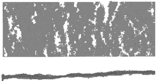
FIG. 1. CT derived fracture geometry used to create the flow models. White zones are regions of no-flow, where the fracture walls touch.
