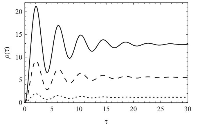
FIG. 7. Mean-square displacement  $\rho$  vs time lag  $\tau$  in the case of external noise (i.e.,  $k_B T/\omega^2 = 0$ ). System parameter values:  $\omega = 0$ ,  $A_0 = 1$ ,  $D_1 = 0.01$ ,  $D = 0.5$ ,  $\gamma = 3.5$ ,  $\alpha = 0.22$ , and  $\tau_c = 0.1$ . Solid line,  $\Omega = 1.5$ ; dashed line,  $\Omega = 1.3$ ; dotted line,  $\Omega = 2.0$ .
