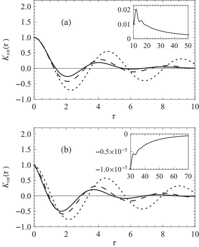
FIG. 2. Normalized autocorrelation functions  $K_{xn}(\tau)$  and  $K_{vn}(\tau)$  vs the time lag  $\tau$  in the case of external noise (i.e.,  $T = 0$ ). System parameter values:  $\omega = 1$ ,  $\gamma = 1.6$ ,  $\alpha = 0.5$ ,  $D = 0.3$ , and  $D_1 = 0.1$ . Solid line,  $\tau_c = 0.01$ ; dashed line,  $\tau_c = 0.1$ ; dotted line,  $\tau_c = 1$ . The insets depict the behavior of  $K_{xn}$  and  $K_{vn}$  at large values of  $\tau$ ;  $\tau_c = 0.01$ .
