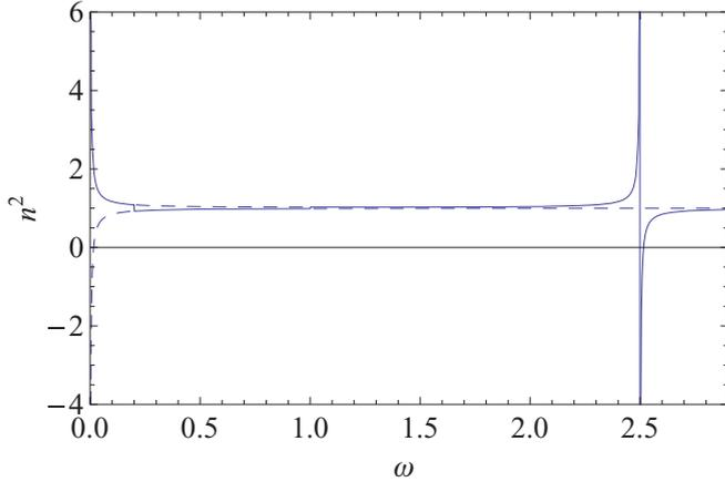
FIG. 1. (Color online) Dispersion curves are plotted for parallel propagation  $\theta = 0$  for  $\omega_p/\Omega_e = 0.2$  and  $\Omega_m/\Omega_e = 1.5$ . The two solutions of the dispersion equation are shown as the solid and dashed curves.
