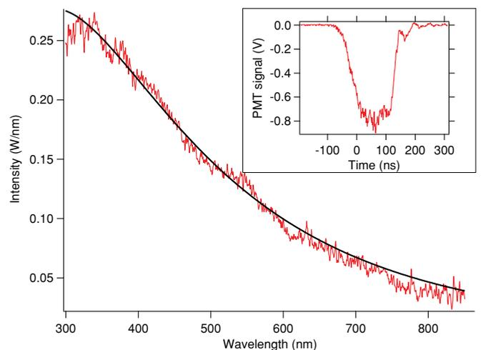
FIG. 3. (Color online) Diagram showing a representative spectrum compiled from 4 separate flashes. The fit is a 10 200-K black body spectrum with an emission radius of 125  $\mu\text{m}$ . This radius is sufficiently close to the measured radius for us to conclude that the emission is that of a black body. The inset is a typical PMT trace.
