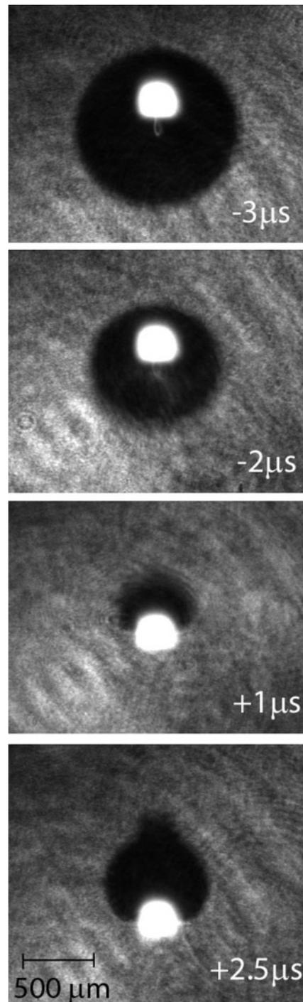
FIG. 5. A series of backlighting images near collapse. Each photo is a 30-ns backlighting exposure. Sonoluminescence is exposed in every photo. In each photo the time relative to the sonoluminescence signal is given. The jet is clearly starting to emerge in the final photo.
