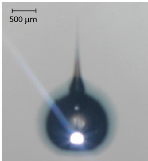
FIG. 4. (Color online) A backlit photograph of the jet formed during collapse. The bright blue light near the bottom of the bubble is the sonoluminescence. The strobe time is  $50 \mu\text{s}$ , which causes considerable blurring in the bubble wall.
