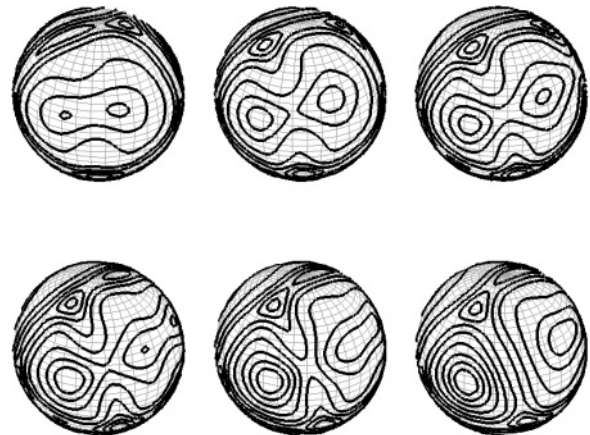
FIG. 8. Contour plots of the radial velocity for Ra = 23\,500 at time points t_0 = 4.13 , t_1 = t_0 + 0.4\tau , t_2 = t_0 + 0.8\tau , t_3 = t_0 + 0.9\tau , t_4 = t_0 + 0.95\tau , and t_5 = t_0 + \tau from left to right and from top to bottom.
