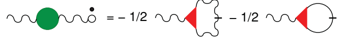
FIG. 1. (Color online) Diagrammatic representation of the flow equation which determines the flow of the order parameter and which arises from the vanishing flow of the one-point vertex [28]. Wavy lines correspond to G_{ab} propagators and solid lines to G_{hh} . Lines with a dash correspond to single-scale propagators. The small open circle with a dot denotes a derivative of the order parameter with respect to \Lambda .
