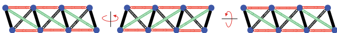
FIG. 4. (Color online) If K_{++} = K_{--} , the structure is mapped into itself by the symmetry operations shown in this diagram.
