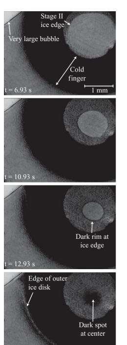
FIG. 3. These images show a sequence of snapshots of stage II solidification for a sample of 142-nm particles. In areas where stage II ice has formed, the sample appears darker. The stage II ice edge is marked by a dark rim of particles being pushed ahead of the ice, which form a dark spot at the center upon complete solidification.
