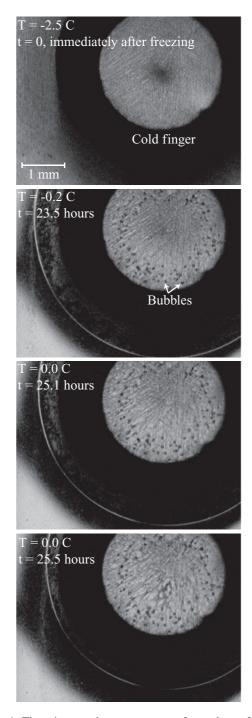
FIG. 4. These images show a sequence of snapshots of a frozen solution of 32-nm particles over time with the sample ages and temperatures indicated. The small dark spots near the cold finger are air bubbles. Because the water was not degassed before freezing, air gradually exolves from the ice.
