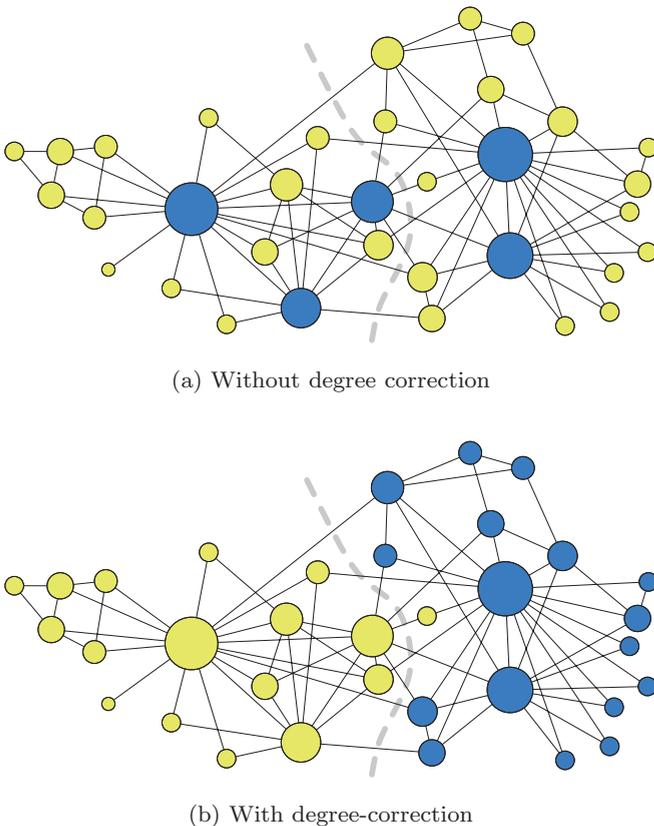
FIG. 1. (Color online) Divisions of the karate club network found using the (a) uncorrected and (b) corrected blockmodels. The size of each vertex is proportional to its degree and the shading reflects inferred group membership. The dashed line indicates the split observed in real life.
