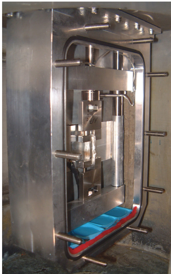
FIG. 1. (Color online) Photograph of a silk sample (white fiber bundle in the center of the image) inside the humidity chamber for in situ tensile testing mounted inside the sample bay of the time-of-flight spectrometer IN6. The chamber is shown with the front cover removed. The force sensor is visible as a cylindrical metal structure on the upper center of the photograph with the signal cable arriving from the right. The neutron beam impinges on the sample horizontally, arriving from the right edge of the photograph. The blue plastic troughs at the bottom of the chamber contain pure water or saturated salt solutions, respectively, to define the humidity inside the chamber. The edge-to-edge distance between the steel hooks holding the fiber bundle is 3 cm.
