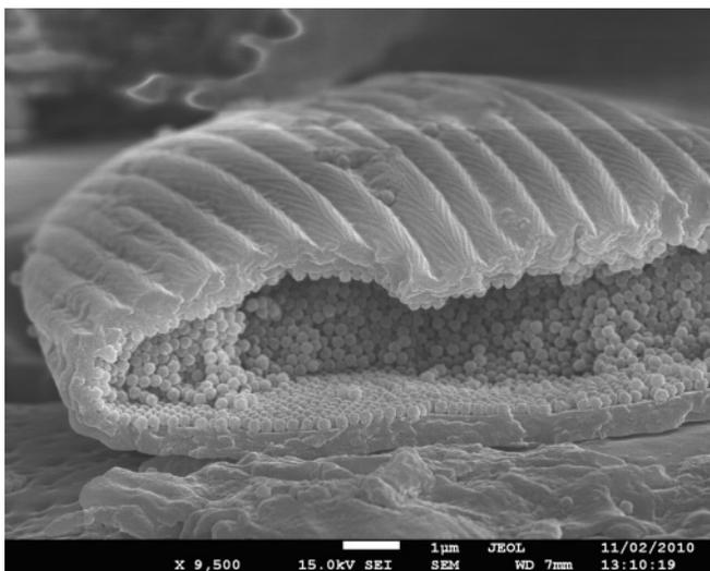
FIG. 5. Electron microscope image of a broken scale randomly selected on one of the elytra of the longhorn *Pseudomyagrus waterhousei*. The scale has an external cortex filled with a regular arrangement of monodispersed chitin spherules. (scale bar 1 micron).
