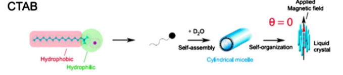
FIG. 1. (Color online) The self-assembly of CTAB molecules into a micelle, the self-organization of those micelles into a liquid-crystal nematic phase, and subsequent alignment by a magnetic field.
