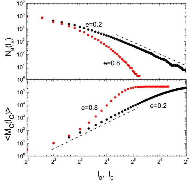
FIG. 2. (Color online) The upper panel shows the number of covering boxes as a function of box size  $l_B$  for the SHM model with  $e=0.2$  (circle) and  $0.8$  (square). The lower panel shows the average number of nodes in a box of size  $l_C$  as a function of  $l_C$  for the same networks. Dashed lines are a guide to the eyes with the slopes of  $d_B=3.19$  and  $d_C=3.44$ .
