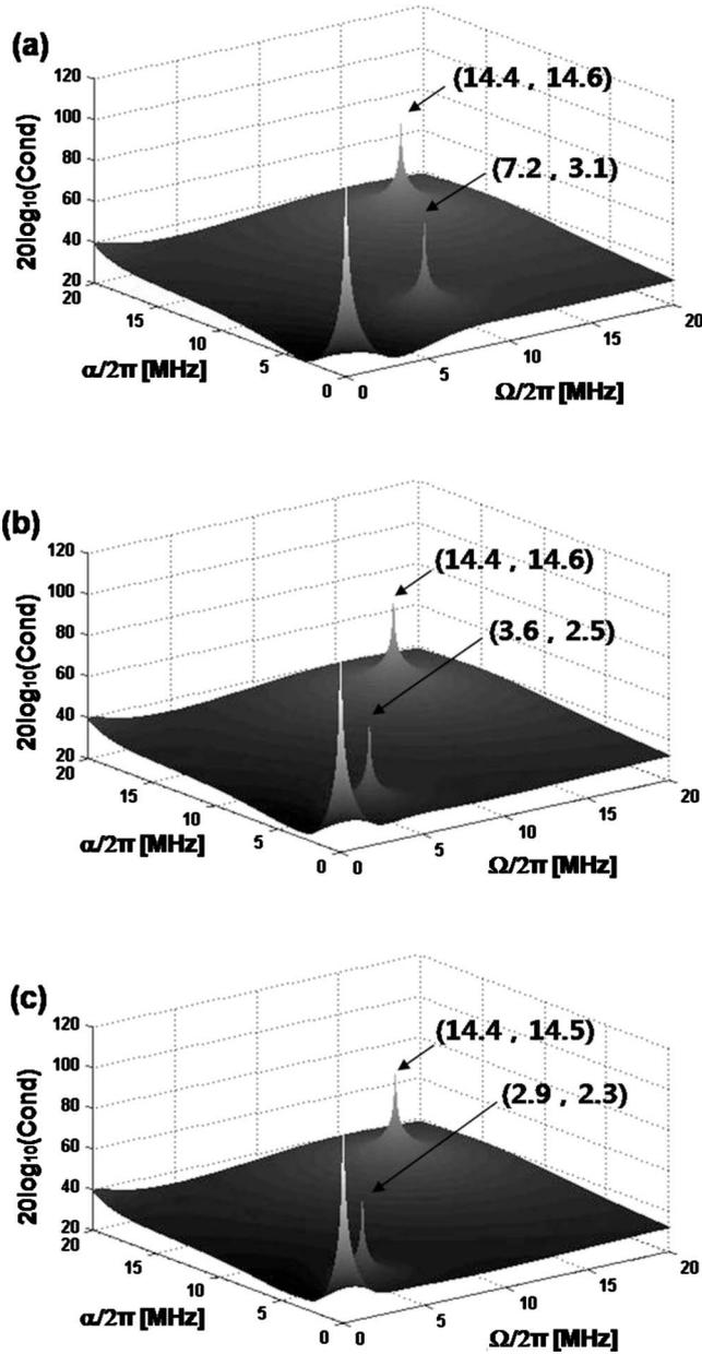
FIG. 1. Condition number of the system matrix as a function of frequency  $\Omega/2\pi$  and decay rate  $\alpha/2\pi$  for the case of *E. coli*: (a)  $T_0=7.50 \times 10^{-2}$  N/m, (b)  $T_0=0.1K_A$ , and (c)  $T_0=0$ .
