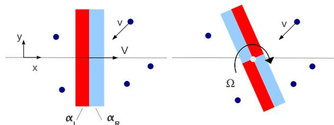
FIG. 1. (Color online) Granular motors. Left: the asymmetric piston; right: the chiral rotor. Both motors are constructed from materials with different coefficients of restitution and are immersed in a bath of thermalized particles. The asymmetric piston acquires a net drift velocity along a line, while the chiral rotor acquires a net rotation around its axis.
