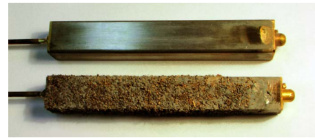
FIG. 8. (Color online) A photograph of two brass cylinders of square cross section 2 \times 2 \text{cm}^2 . The surface of the lower one was roughened by soldering small brass shavings to it; this surface was then electrochemically cleaned and gold plated.
