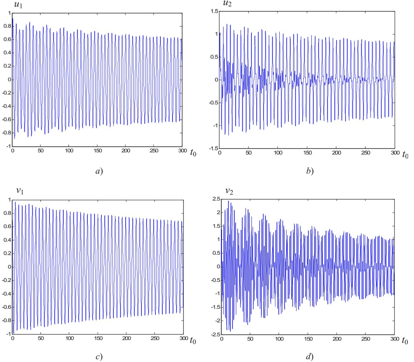
FIG. 16. (Color online) Temporal evolution of displacements and velocities in the dissipative system: (a)  $u_1$ , (b)  $u_2$ , (c)  $v_1$ , (d)  $v_2$ .
