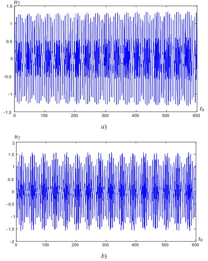
FIG. 13. (Color online) Displacement  $u_2$ : (a): numerics, (b): theory;  $\varepsilon=0.0675$ ,  $c_0=6$ ,  $k_0=4$ ,  $V_0=1$ .
