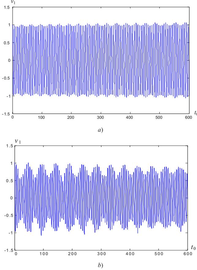
FIG. 14. (Color online) Velocity  $v_1 = du_1/dt_0$ : (a) numerics, (b) theory;  $\varepsilon=0.0675$ ,  $c_0=6$ ,  $k_0=4$ ,  $V_0=1$ .
