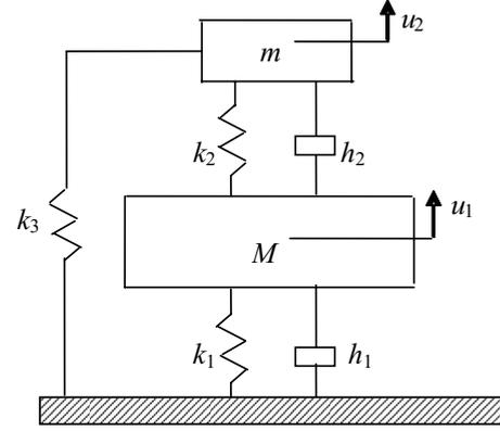
FIG. 10. Scheme of a 2DOF system.
