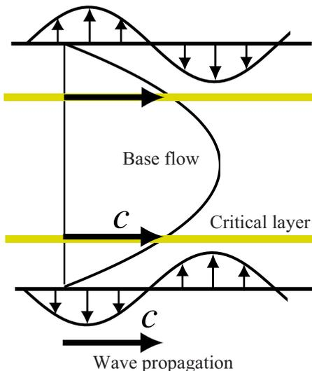
FIG. 5. (Color online) Schematic of a critical layer.
