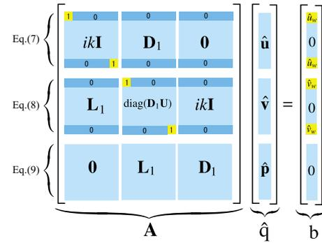
FIG. 26. (Color online) Schematic of the system matrix equation with the boundary conditions. The blocks correspond to the discretized version of Eqs. (7)–(9).
