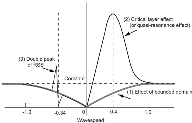
FIG. 8. Schematic of the dimensionless influence layer thickness: thick gray line, effect of bounded domain only; thin black line, actual behavior.
