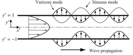
FIG. 1. Flow geometry and schematic of control input.
