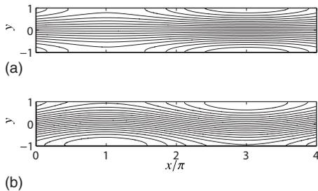
FIG. 20. Streamline by the wave of (a) varicose mode and (b) sinuous mode ( $k=0.5$ ,  $c=-1.5$ , and  $Re=2000$ ).
