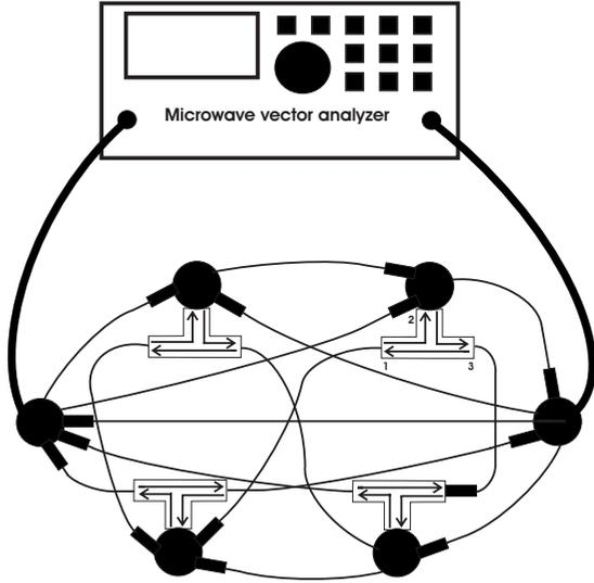
FIG. 2. The scheme of the experimental setup for measuring the two-port scattering matrix  $\hat{S}$  of microwave networks with broken time reversal symmetry. The network additionally to the attenuators contains four microwave circulators. The microwave circulators are enlarged to show the input ports and the directions of traveling waves. The measurements were performed in the frequency window: 7–14 GHz.
