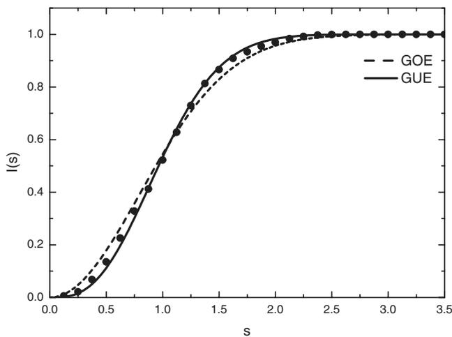
FIG. 3. The integrated nearest-neighbor distribution  $I(s)$  obtained for microwave networks with broken TRS (full circles). The measurements were performed in the frequency range 7–9 GHz. The distribution  $I(s)$  was averaged over 20 microwave network configurations. The experimental distribution is compared to the theoretical predictions for GOE (broken line) and GUE (full line).
