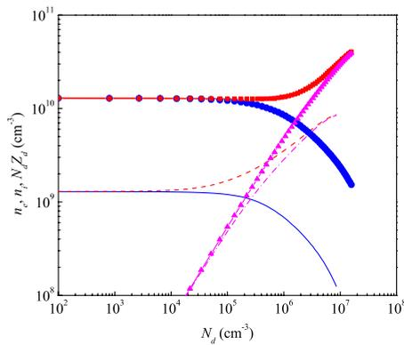
FIG. 2. (Color online) Charged particle concentration dependencies on dust-particle concentration,  $N_d$ , for different discharge current densities; symbols present results for  $j_z=10 \text{ mA/cm}^2$ : circles for  $n_e$ , squares for  $n_i$ , and triangles for  $N_d Z_d$ , and lines for  $j_z=1 \text{ mA/cm}^2$ : solid line for  $n_e$ , dashed line for  $n_i$ , and dashed dotted line for  $N_d Z_d$ ;  $r_0=1 \mu\text{m}$  and  $N_g=1.75 \cdot 10^{16} \text{ cm}^{-3}$ . Helium.
