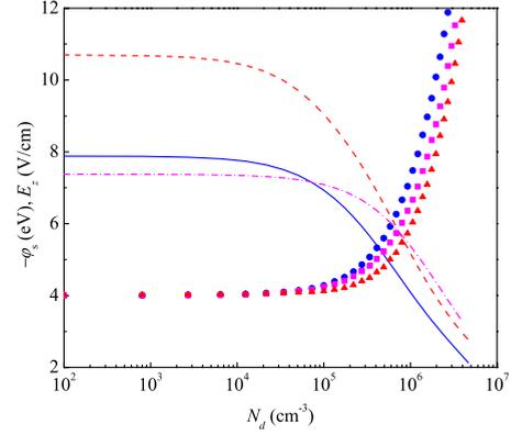
FIG. 5. (Color online) Dust-particle surface potential ( $\varphi_s$ , lines) and axial electric field (symbols) dependencies on dust-particle concentration,  $N_d$ , for different buffer gases: solid line and circles for helium; dashed line and triangles for neon; dashed dotted line and squares for argon;  $r_0 = 1 \mu\text{m}$ ,  $N_g = 1.75 \cdot 10^{16} \text{ cm}^{-3}$ , and  $j_z = 1 \text{ mA/cm}^2$ .
