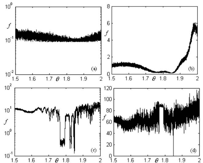
FIG. 6. The graphs of the objective function for the time series of chaotic system (9) with Gaussian noise of zero mean, 0.01 variance, and 0.1 amplitude and here  $\theta=1.85, x_0=0.3, h=0.001$ : (a)  $W=5$ , (b)  $W=10$ , (c)  $W=20$ , and (d)  $W=100$ .
