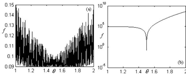
FIG. 4. The graphs of the objective function for the time series of incipiently unstable system (8) with Gaussian noise of zero mean, 0.01 variance, and 0.1 amplitude and here  $\theta=1.5, x_0=0.3, h=0.001$ : (a)  $W=2$ ; (b)  $W=20$ .
