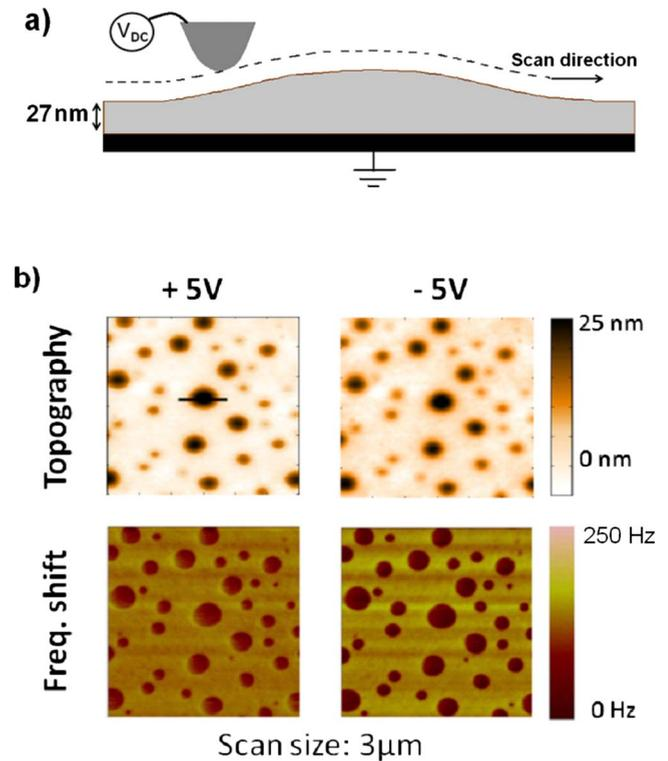
FIG. 2. (Color online) (a) Typical topographic profile of PVAc islands in a PS matrix. Both tip and polymer film are represented at the same scale. The dash line represents the tip motion during the second scan. (b) Topography and frequency shift measured by the double pass method at +5 and  $-5$  V on the PVAc/PS films. The black line corresponds to the profile appearing in (a).
