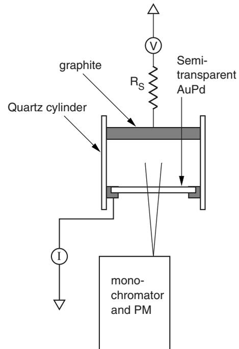
FIG. 1. Schematic of the drift tube, monochromator, photomultiplier, and electrical circuit for the discharge.
