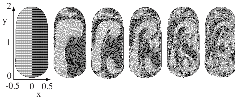
FIG. 6. Evolution of passive tracers for a drop forced in a sinusoidal channel simulated by time varying shearing. Each figure is a snapshot taken after one full period of the imposed shear. The governing parameters here are Re = 1 , Ca = Re/We = 0.02 , \lambda = 1 , and \rho_c / \rho_d = 1 . The upper portion of the drop is its front, the lower portion is its back.
