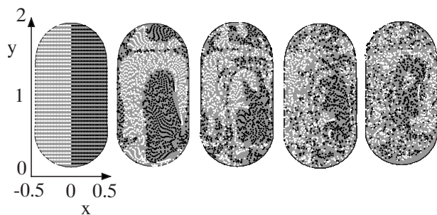
FIG. 9. Evolution of passive tracers for a drop forced in a sinusoidal channel simulated by time varying shearing. Each figure is a snapshot taken after one full period of the imposed shear. The governing parameters here are Re=1 , Ca=0.004 , \lambda=1 , and \rho_c/\rho_d=1 . The mixing pattern is similar to that for Ca=0.02 but evolves faster. The upper portion of the drop is its front; the lower portion is its back.
