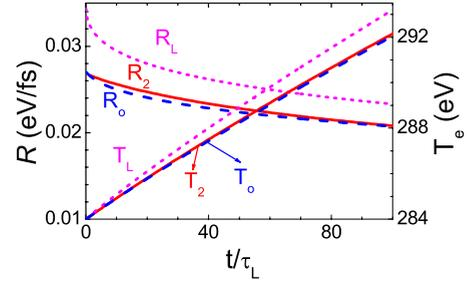
FIG. 4. (Color online) The absorption rates  $R$  and plasma temperatures  $T_e$  updated by 2VFP code (solid line), Langdon's IB operator (short dashed line), and our IB operator (dashed line). The plasma and laser parameters are electron density of  $1.5 \times 10^{19}$  cm<sup>-3</sup>, initial temperature of 284 eV, ionization state of  $Z_i = 7$ , laser wavelength of 1.054  $\mu\text{m}$ , and intensity of  $6.3 \times 10^{14}$  W/cm<sup>2</sup>.
