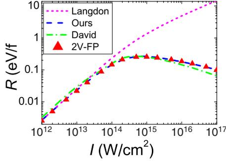
FIG. 2. (Color online) The absorption rates  $R$  averaged over the first four laser cycles as functions of laser intensity obtained from 2VFP code (triangle), Langdon's IB operator (short dashed line), our IB operator (dashed line), and David's fitted formula (6) in Ref. [29] from molecular-dynamic method (dash-dotted line). The plasma and other laser parameters are as in Fig. 1.
