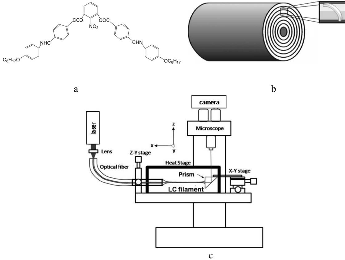
FIG. 1. (a) Illustration of the molecular structure of the bent-core liquid-crystal material 2-nitro-1,3-phenylene-bis[4-(4-8-alkoxyphenyliminomethyl) benzoates (Ref. [4]). (b) The smectic layer arrangement in the filament (Ref. [7]). (c) Schematic of the experimental apparatus.
