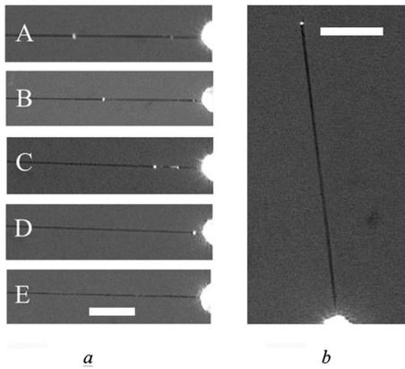
FIG. 3. (a) Translation of a defect (position of defect is a bright spot in the filament) in a newly pulled filament vs time. The time in between images A–E is  $\sim 4$ – $5$  min. (b) Free-standing filament of bent-core mesogens in the Cr phase, held at  $35^\circ\text{C}$ . White bars indicate  $50\ \mu\text{m}$  length.
