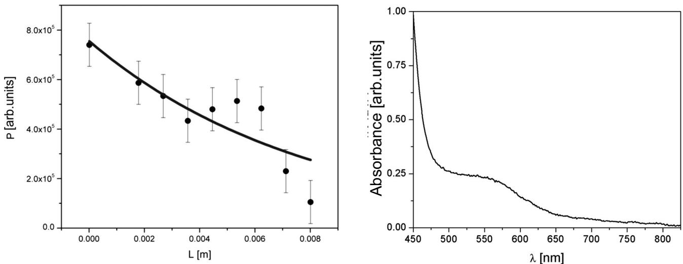
FIG. 4. (a) Transmitted power vs filament length at  $175^\circ\text{C}$  at  $532\ \text{nm}$  of a  $6.5\ \mu\text{m}$  fiber. The experimental data were fitted by an exponential. (b) Absorbance vs wavelength measured by a Ocean Optics spectrophotometer,  $5\ \text{mm}$  path-length cuvette where  $2.1\ \text{mg}$  of 2-nitro-1,3-phenylene-bis[4-(4–8-alkyloxyphenyl)iminomethyl] benzoates] was mixed into  $0.5\ \text{ml}$  of ethyl acetate.
