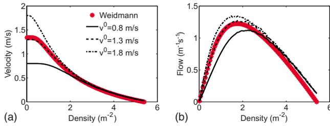
FIG. 5. (Color online) Fundamental diagrams and velocity-density relations generated by Eq. (1), for different free speeds  $v^0$ . Note how they all converge for large densities. As a comparison, the empirical fit curve by Weidmann [3] is shown.
