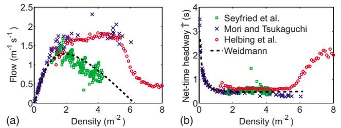
FIG. 3. (Color online) (a) flow as a function of density for data from a number of empirical studies. (b) the net-time headways  $\hat{T}$  as a function of density  $\rho$ .  $\hat{T}$  is most often bounded by a constant lower value of about 0.5 s. In the data of Ref. [2], however, there is a transition for high densities where  $\hat{T}$  suddenly increases. The data sets are the same as used in Ref. [2], i.e., the data from (Helbing *et al.*) correspond to *local* densities and flows.
