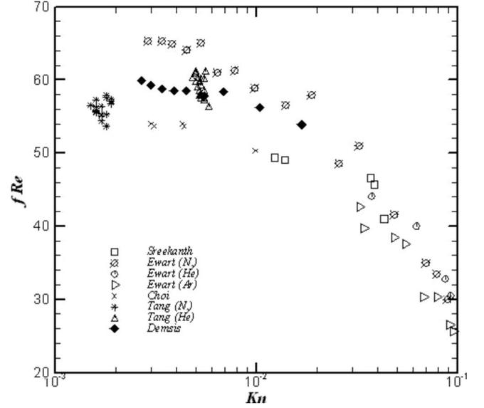
FIG. 3. Friction factor times Reynolds number as a function for Knudsen number—present data and comparison with literature. The friction factor for Sreekanth was calculated based on data in his paper.
