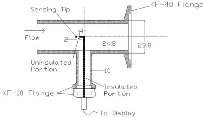
FIG. 5. Schematic of the bended thermocouple.
