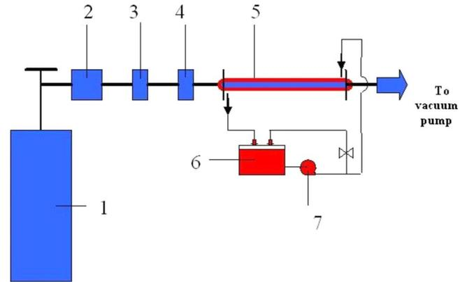
FIG. 1. (Color online) Layout of the experimental setup: 1-nitrogen cylinder; 2-pressure regulator; 3-particle filter; 4-mass flow controller; 5-counter flow tube-in-tube heat exchanger; 6-hot water tank; and 7-water pump.
