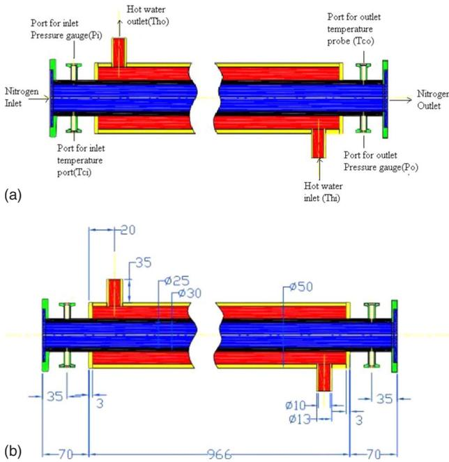
FIG. 2. (Color online) (a) Schematic of the tube-in-tube heat exchanger and (b) schematic with dimensions (in mm) of the heat exchanger.
