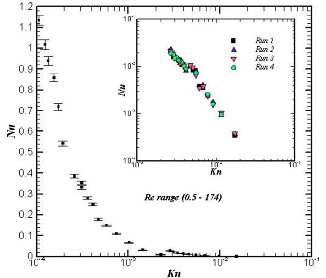
FIG. 4. (Color online) Variation of Nusselt number as a function of Knudsen number; inset shows variation of Nusselt number as a function of Knudsen number for four different runs (in the slip regime), showing repeatability in the measurements. Note that the results have been plotted on a log-log scale to highlight the low values of Nusselt number and depict the trend clearly in the slip regime.
