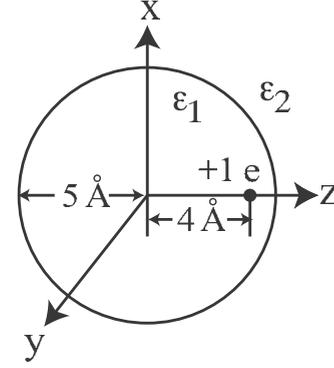
FIG. 1. The geometry of the model problem: a dielectric sphere of radius 5 Å, centered at the origin, with dielectric constant  $\epsilon_1$  is embedded in a homogeneous dielectric medium of dielectric constant  $\epsilon_2$ . A single discrete point charge of value  $+1e$  is located at  $(0, 0, 4 \text{ \AA})$ .
