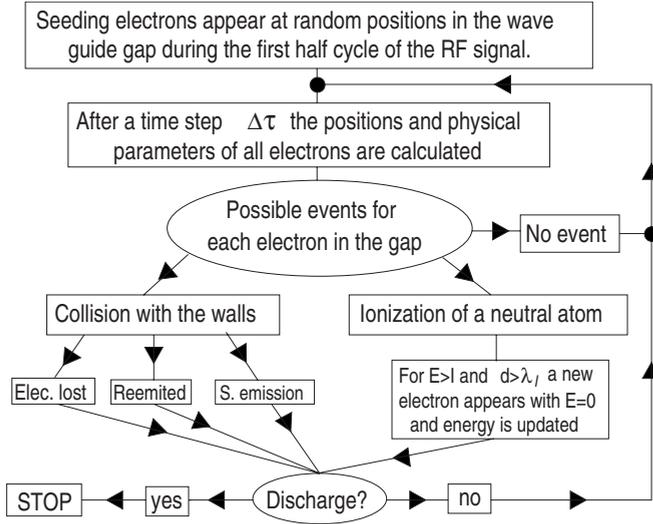
FIG. 3. Structure of the numerical simulations.
