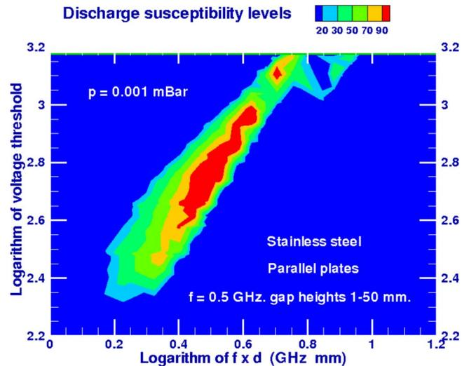
FIG. 5. (Color online) The rf voltage thresholds as a function of  $f_w D$  for the low pressure electron multipactor. The decimal logarithm is employed in both axes.
