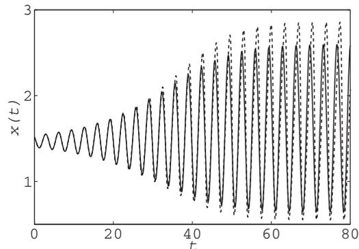
FIG. 2. The comparison of the approximate (solid line) and exact (dashed line) solutions for the substrate concentration in the local system. The parameters:  $w=2$ ,  $\nu=2.73$ .
