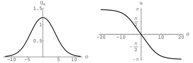
FIG. 5. Tensile macrostrain wave and corresponding microstrain wave with the velocities from the interval  $c_L^2 + c_0^2 < V^2$ ,  $V^2 > c_l^2$ .
