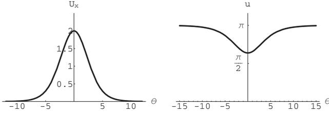
FIG. 7. Tensile macrostrain wave and corresponding microstrain wave in the interval  $c_L^2 < V^2 < c_L^2 + c_0^2$ ,  $V^2 > c_l^2$ .
