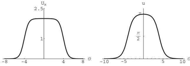
FIG. 3. “Fat” compression macrostrain wave and corresponding wave of microstrain when  $V^2 \rightarrow c_L^2 - c_0^2$ .
