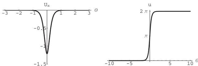
FIG. 1. Compression macrostrain wave and corresponding wave of microstrain in the interval  $c_L^2 + c_0^2 < V^2 < c_L^2$ .
