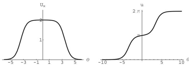
FIG. 4. “Fat” macrostrain compression wave and corresponding microstrain wave for  $V^2 \rightarrow c_L^2 - c_0^2$ .
