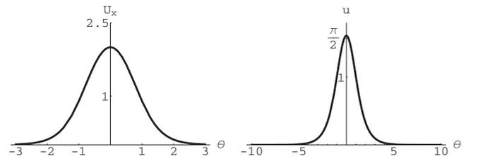
FIG. 2. Compression macrostrain wave and corresponding wave of microstrain in the interval  $c_L^2 - c_0^2 < V^2 < c_L^2$ ,  $V^2 < c_L^2$ .
