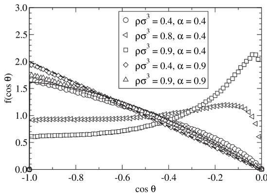
FIG. 8. The distributions of collisional angles for (i)  $\rho\sigma^3=0.4$  and  $\alpha=0.4$  (circles), (ii)  $\rho\sigma^3=0.8$  and  $\alpha=0.4$  (left triangles), (iii)  $\rho\sigma^3=0.9$  and  $\alpha=0.4$  (squares), (iv)  $\rho\sigma^3=0.4$  and  $\alpha=0.9$  (diamonds), and (v)  $\rho\sigma^3=0.9$  and  $\alpha=0.9$  (up triangles). The dashed line is for elastic hard spheres and the solid line is from a DSMC simulation of  $\rho\sigma^3=0.9$  and  $\alpha=0.4$ .
