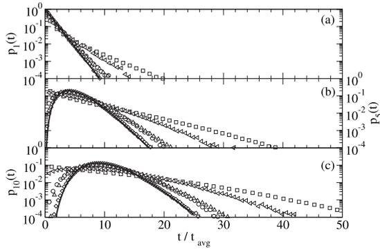
FIG. 10. Distributions of time between (a) one collision, (b) five collisions, and (c) ten collisions in sheared inelastic hard spheres with (i)  $\rho\sigma^3=0.4$  and  $\alpha=0.4$  (circles), (ii)  $\rho\sigma^3=0.9$  and  $\alpha=0.4$  (squares), (iii)  $\rho\sigma^3=0.4$  and  $\alpha=0.9$  (diamonds), and (iv)  $\rho\sigma^3=0.9$  and  $\alpha=0.9$  (triangles). The solid line is for a Poisson process.
