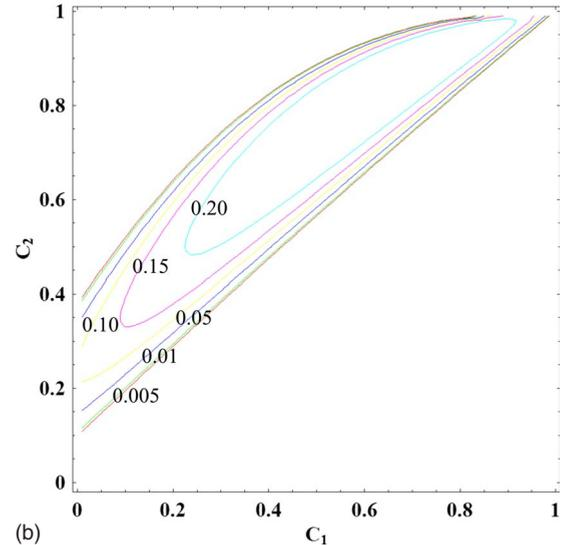
FIG. 6. (Color online) The three-dimensional graph and isoline map of efficiency  $\eta$  varying with the variables  $C_1$  and  $C_2$  for the parameters  $G=10g$ ,  $T_H=2.0 \times 10^{-5}$  K, and  $T_L=1.0 \times 10^{-5}$  K.
