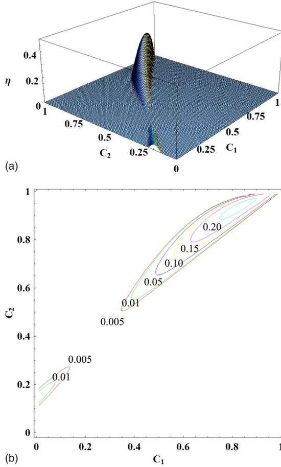
FIG. 7. (Color online) The three-dimensional graph and isoline map of efficiency  $\eta$  varying with the variables  $C_1$  and  $C_2$  for the parameters  $G=30g$ ,  $T_H=2.0 \times 10^{-5}$  K, and  $T_L=1.0 \times 10^{-5}$  K.
