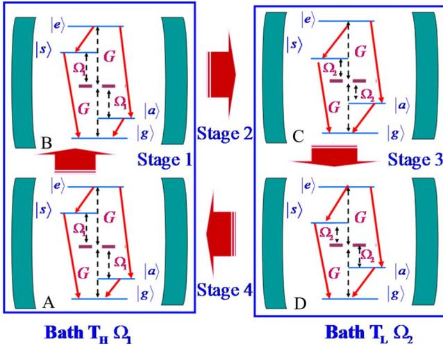
FIG. 4. (Color online) A schematic diagram of a thermal entangled quantum Otto engine based on two two-level atoms of quantum system. The process from A to B (C to D) is the isothermal expansion (compression) process, in which the working substance is put in contact with the high (low)-temperature heat bath. The processes from B to C and from D to A are two adiabatic processes.
