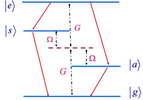
FIG. 1. (Color online) Collective states of two two-level identical atoms. The energies of the symmetric and antisymmetric states are shifted by the dipole-dipole interaction  $\Omega$ . The arrows indicate possible one-photon transitions.
