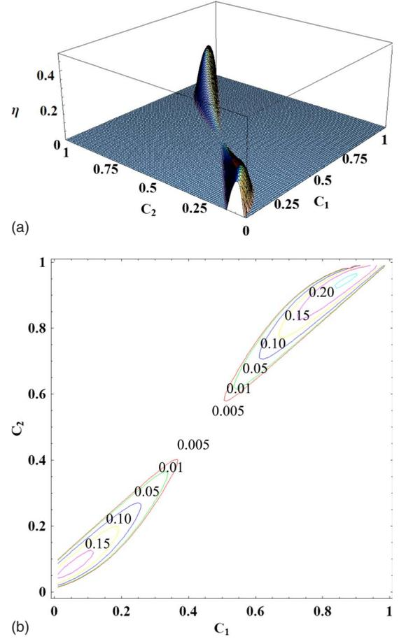
FIG. 8. (Color online) The three-dimensional graph and isoline map of efficiency  $\eta$  varying with the variables  $C_1$  and  $C_2$  for the parameters  $G=50g$ ,  $T_H=2.0 \times 10^{-5}$  K, and  $T_L=1.0 \times 10^{-5}$  K.
