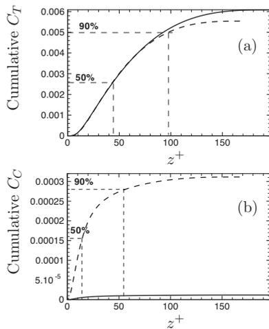
FIG. 2. Cumulative contribution of Reynolds stress (a) and of compressible terms (b) to skin friction for Mach number  $M=0.4$  (—) and  $M=2$  (- -).
