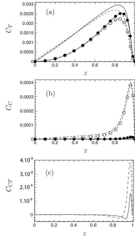
FIG. 3. Reynolds stress terms (a), compressible terms (b), and compressible/turbulent terms (c) contribution to skin friction for Mach number  $M=0.4$  (—) and  $M=2$  (- -), and its weighted contributions (with circle).
