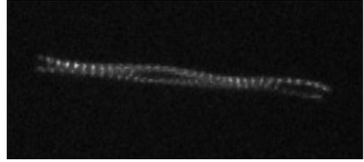
FIG. 6. Coordinate tracing for oblong ellipsoid shaped particle; ellipsoid axis ratio is 1:2. Particle rotates with frequencies  $\omega = 6600$  rad/s and  $\Omega = 190$  rad/s. Conditions: Ne,  $p=0.7$  Torr,  $i = 2.5$  mA. Horizontal size of images is 190  $\mu\text{m}$ .
