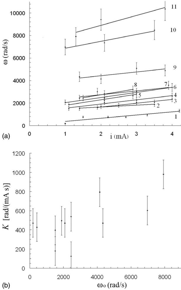
FIG. 5. (a) Dependence of angular velocity on discharge current for several particles (1–11). Conditions: Ne,  $p=0.7$  Torr. 10% error is caused by dead time between frames. (b) Dependence of coefficient  $K$  on frequency  $\omega_0$  at  $i=1.5$  mA for particles of (a).
