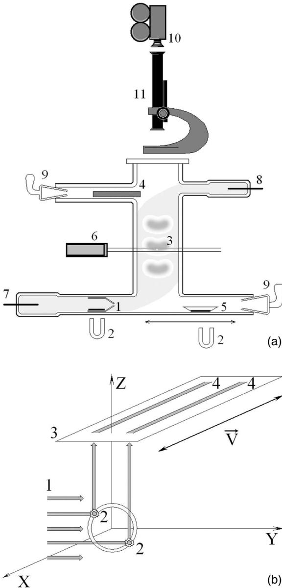
FIG. 1. (a) Experimental setup. (1) movable diaphragm, (2) magnet, (3) stratum, (4) container with microspheres, (5) dust collector, (6) laser, (7) cathode, (8) anode, (9) vacuum ports, (10) video camera, and (11) microscope. (b) Formation of coordinate tracing. (1) laser beam, (2) particle surface areas scattering light to optical system, (3) charge-coupled device (CCD) matrix, (4) image of moving particle on the CCD matrix. Arrow shows the direction of CCD matrix shift.
