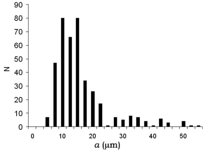
FIG. 2. Particle size distribution. Conditions: air,  $p=0.2$  Torr,  $i=1$  mA, and  $a$  is the radius of the 402 particles sphere.
