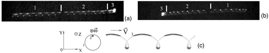
FIG. 3. (a), (b) Examples of coordinate tracing. Images of three consecutive frames. Gaps in a trajectory are caused by “dead time” between frames. (a) Image of particle moves from the left to the right. (b) Image of particle moves from the right to the left. Conditions: Ne,  $p=0.7$  Torr,  $i=1.5$  mA. Horizontal size of both images is 1.1 mm. (c) Explanatory sketch for (a): (1) particle surface, (2) defect, and (3) resulting trajectory (cycloid).
