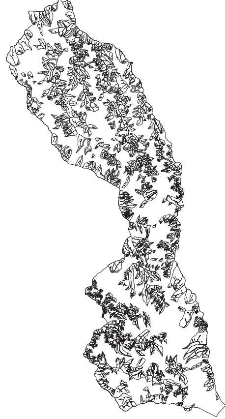
FIG. 5. Hortonian substructures of the Corace river network for the order \omega=2 .
