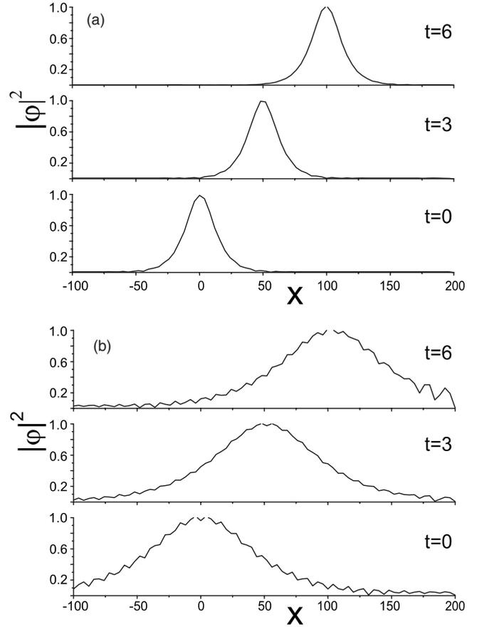
FIG. 2. Numerical time evolution of a bright soliton under the action of Eq. (28) for  $\theta=0.1$  (a) and  $\theta=0.9$  (b). Other parameters are taken as follows:  $S=10$ ,  $B=100$ ,  $J=1$ , and  $\delta=0.1$ . It indicates that a bright soliton is excited when  $\theta < \theta_0$ .
