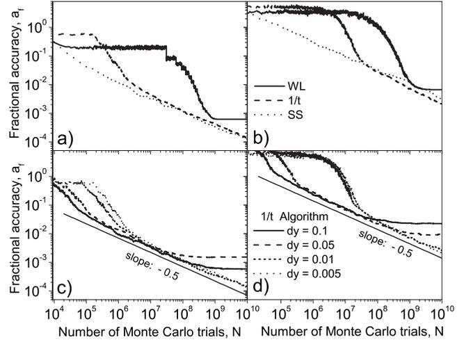
FIG. 1. Dynamical behavior of fractional accuracy  $a_f$  calculated by means of Wang-Landau,  $1/t$ , and simple sampling Monte Carlo integration: (a) for  $I_{1D}$ , with  $dy=0.005$  and  $L=3066$ ; (b) for  $I_{2D}$ , with  $dy=0.005$  and  $L=1213$ . (c) and (d) show the effect of bin width on  $I_{1D}$  and  $I_{2D}$ .
