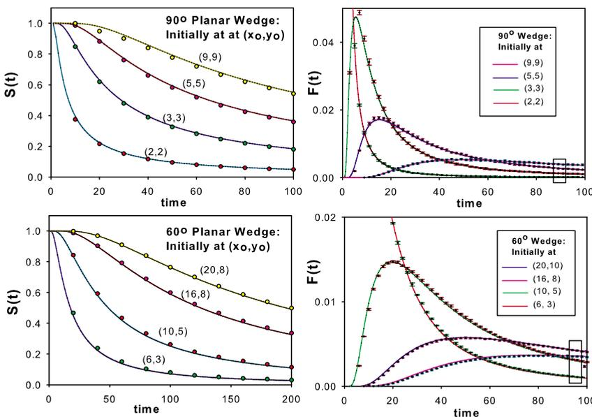
FIG. 4. (Color online) Survival probability and first-passage-time distribution for 1-million walkers initially at  $(x_0, y_0)$ . Solid line refers to the diffusion prediction and the markers are simulation points. The standard deviation is computed over 10 simulation runs.
