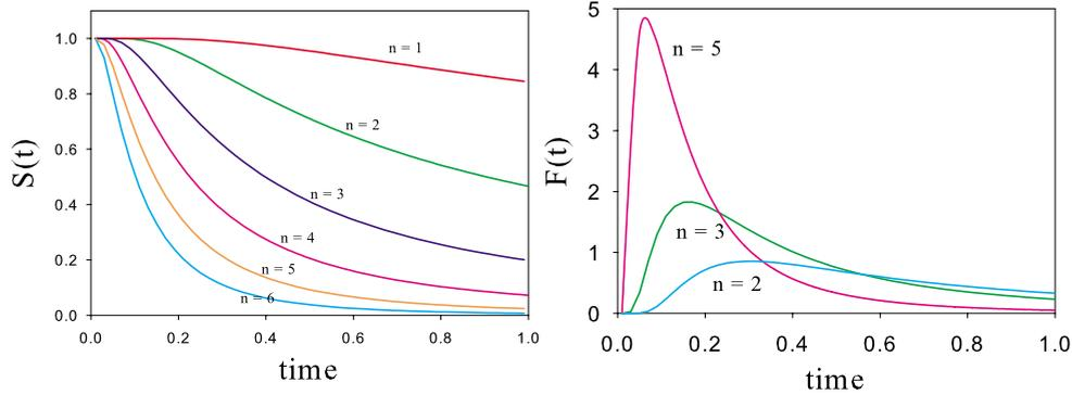
FIG. 3. (Color online) Survival probability and first-passage-time distribution for diffusing particle initially at  $(2 \cos \frac{\pi}{2n}, 2 \sin \frac{\pi}{2n})$  and  $D=1$  for various  $n$ . For the case  $n \in \{1, 2, 3, 5\}$ ,  $S(t)$  comes from an exact expression. For  $n=4, 6$ ,  $S(t)$  was computed numerically.
