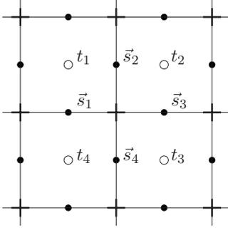
FIG. 1. Part of the square lattice with spin variables (●) and face variables (○) representing the vacancies. The vertices are shown as +. The figure includes the labeling of the variables used in the definition of the local weight  $W(k)$ , when applied to the central vertex in this figure.
