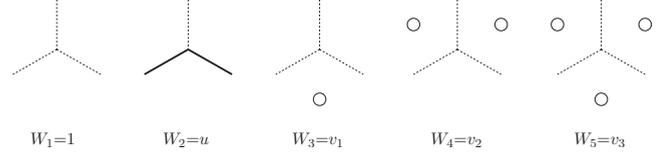
FIG. 4. Vertex weights of the honeycomb  $O(n)$  model with vacancies on the faces. Solid lines represent loop segments and circles the vacancies on the elementary hexagons. A vacancy excludes the six surrounding edges to be visited by a loop. Rotated versions of these vertices have the same weights. The spin variables, which sit on the vertices, play no part in the loop representation.
