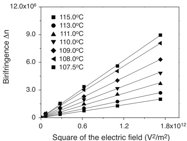
FIG. 2. Induced birefringence  $\Delta n$  as a function of square of the applied field at various temperatures. Solid line is the best fit obtained from a least-mean-squares method.
