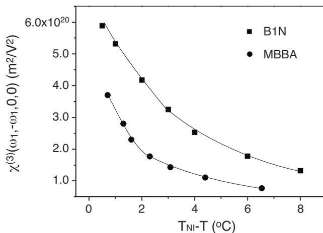
FIG. 4. Variation of nonlinear static susceptibility  $[\chi^{(3)}(\omega_1, -\omega_1, 0, 0)]$  as a function of temperature. Data corresponding to the solid squares are obtained from the present bent-core compound and those of solid circles are from Ref. [18]. Solid lines are drawn as guides to the eye.
