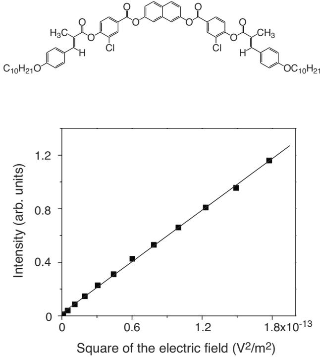
FIG. 1. Transmitted intensity of the modulated signal ( $I_{ac}$ ) as a function of square of the applied field measured at a frequency 2 kHz. The solid line is the best fit obtained from a least-mean-squares method. The sample used is also shown at the top of the figure.
