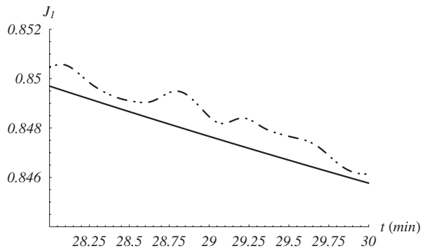
FIG. 5. Behavior of J_1 for Via Parmenide crossing among the dynamic random simulation (double-dot-dashed line) and the fixed simulation with p=0.5 (solid line).
