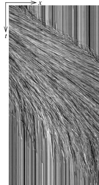
FIG. 10. Space-time plot for a sand avalanche for  $\theta=36.8^\circ$  and  $h_s=0.12 \text{ cm}$ . Image size:  $5.96 \text{ cm} \times 1.43 \text{ s}$  [velocity profile shown in Fig. 20(a)].
