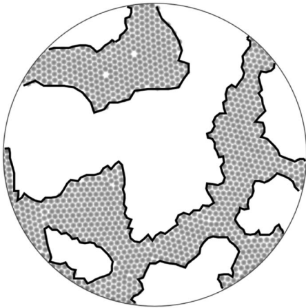
FIG. 8. Definition of boundary length of aggregated nanoparticles: bold black lines.
