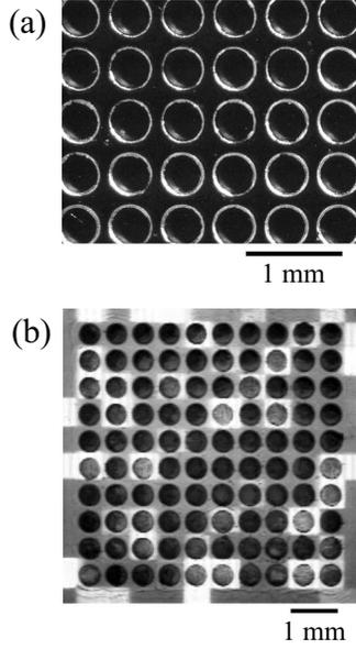
FIG. 1. (a) Patterned microreactor. Each reactor unit has a depth of  $65 \mu\text{m}$  and a diameter of  $430 \mu\text{m}$ . (b) Snapshot of the  $10 \times 10$  microgel array superposed to the illumination pattern with random intensity values at each cell.
