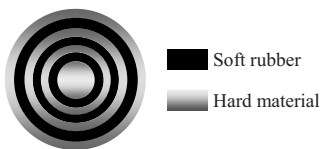
FIG. 1. Representation of the basic unit structure made of a hard cylinder core covered by a multilayer of rubber and steel. N is the number of shells in the coating ( N=6 in this figure).
